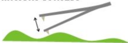
Tapping mode /intermittent contact
