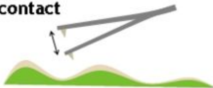
Tapping mode /intermittent contact
