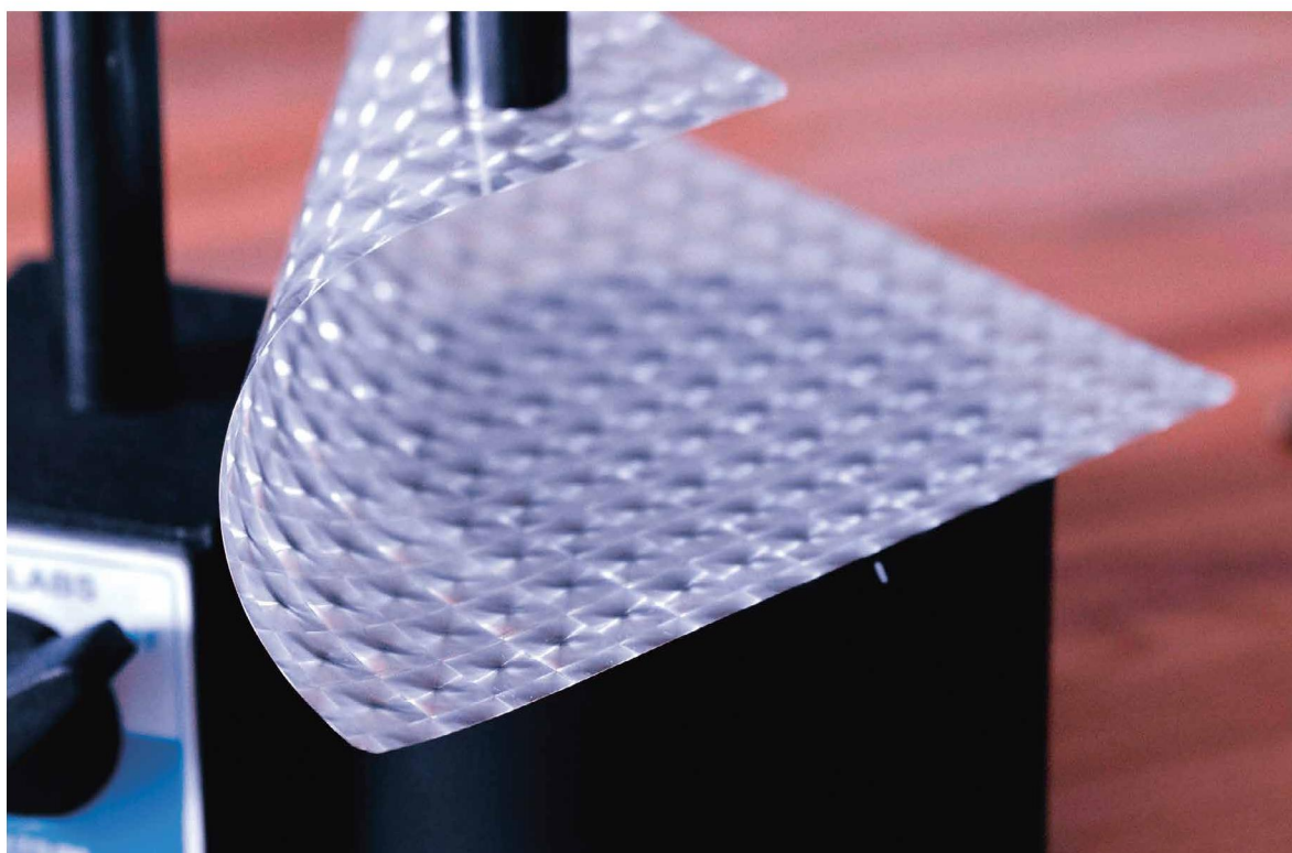
Figure 3: Only an optical foil like this, based on the presented new technology, allows the luminaire design and light distribution shown in figures 1&2
